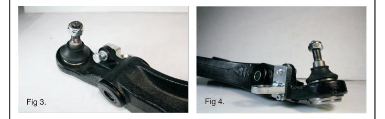
3. Tighten the M10 bolt first to approx. 35-40Nm. Followed by the smaller M6 to approx. 5-6Nm 4. Re-check all bolts after road test.
