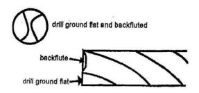
Either of these two methods will permit the swarf to be drawn up the fluting and not cause excessive heat buildup. The urethane will melt, so use a slow RPM drill and a fast feed.
