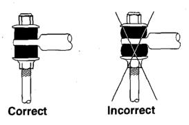
4. Ensuring that the links are vertical tighten U-bolt nuts. Do not over tighten the link bush nuts.
