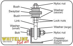
Fig.2. Whiteline pin/eye type link.
