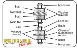
Fig.1. Whiteline double pin type link.
