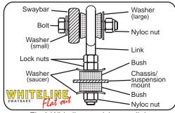
Fig.3 Whiteline eye/pin type link.
