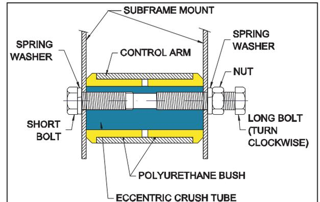
Fig 3 - component assembly.
