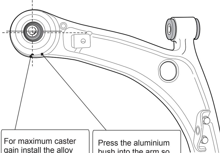
For maximum caster gain install the alloy bush into the arm with the installation indicator notch pointing outward.
