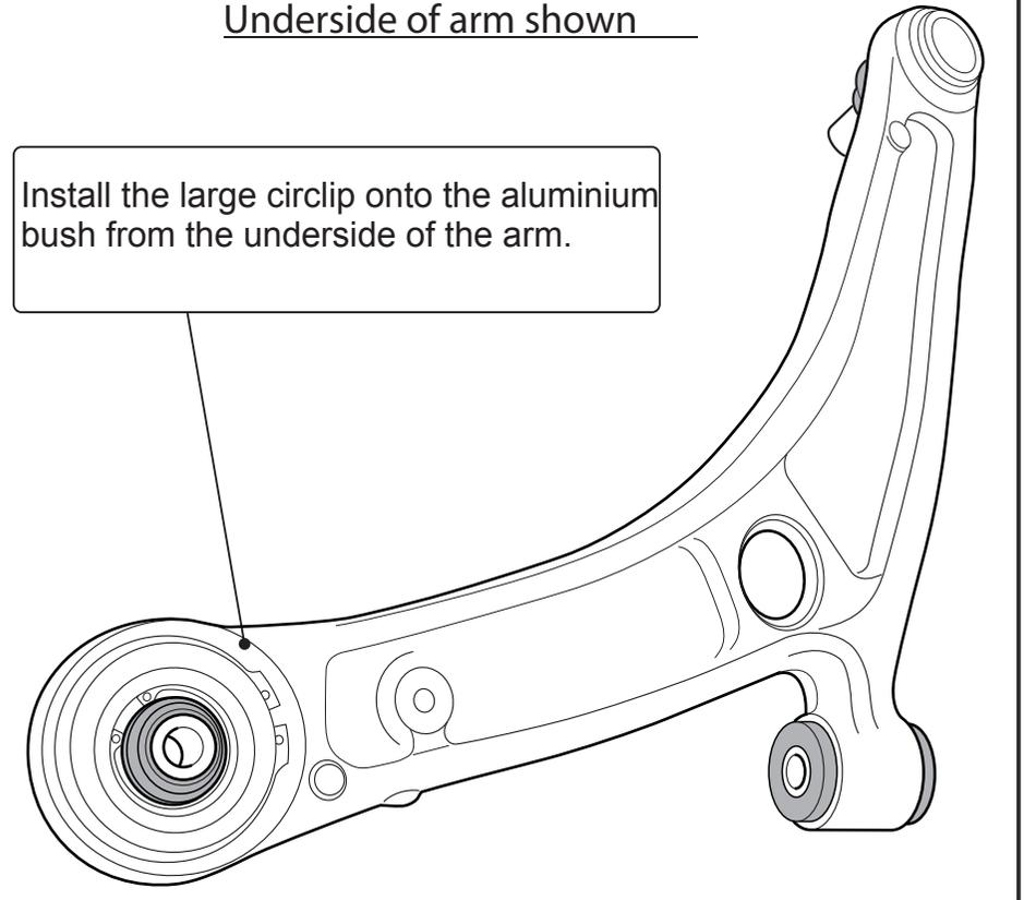
Install the large circlip onto the aluminium bush from the underside of the arm.
