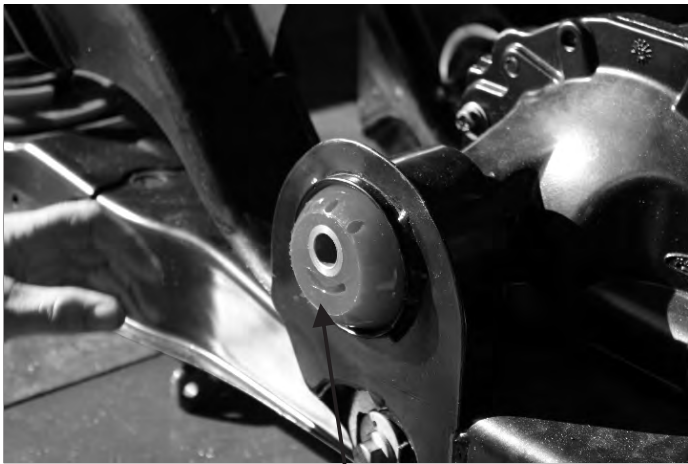
Voiding is to sit directly under bonded tube.
