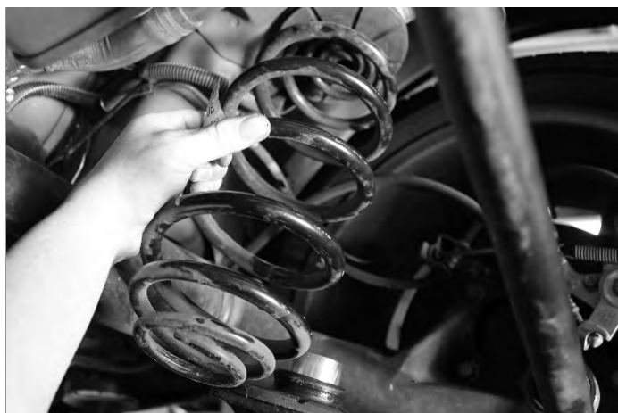
Re fit spring pads and coils
