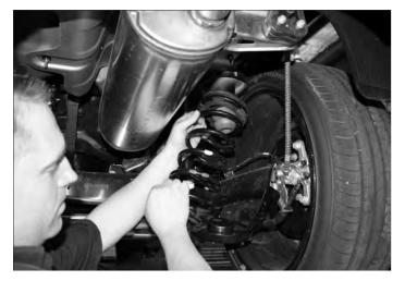
• Once the lower shock mount is unbolted, slowly raise the body - <u>careful to not stretch the brake lines.</u>
